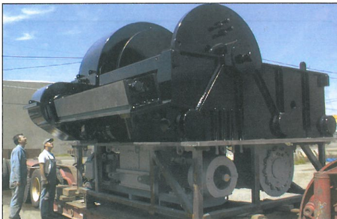
First Class III electric hawser – DESS-52 installed on Crowley's Response, a 7,000hp Voith Tractor tug built a decade ago. This design was based on a one-piece suspended tray deck sill mounted
