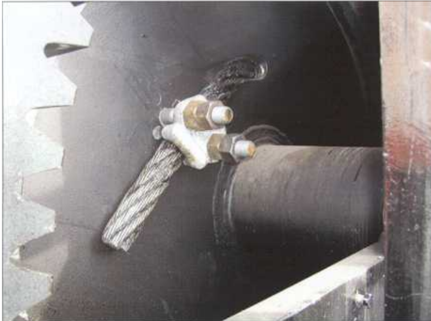
A typical single or double clamp installation to winch side flange. Photo by Barry Griffin.
