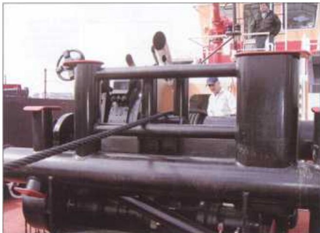
Spooling and tightening the first layer of line on a Markey TES-32, 2-inch wire towing winch. Photo by Barry Griffin.
