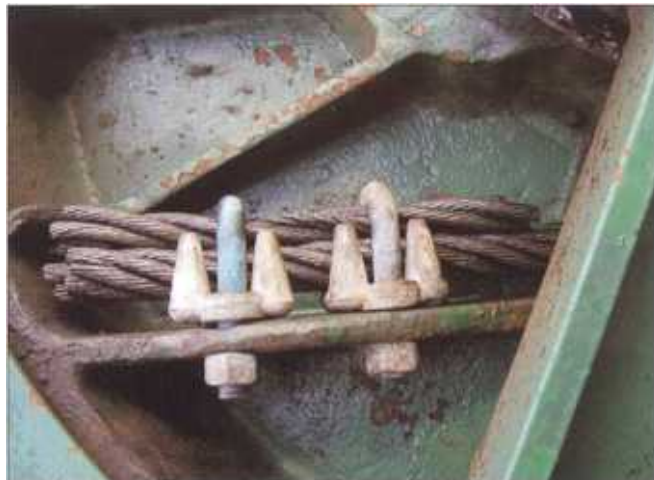
This is a common dead end method shown to have low holding power. Photo by Barry Griffin.
