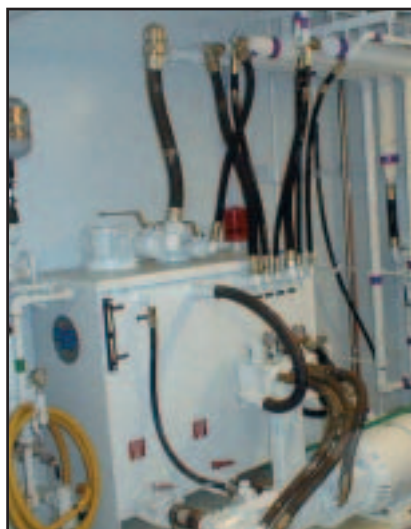
A Markey 40 hp hydraulic power unit delivers about 28 to 30 useful horsepower to the hawser.
